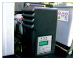
On-board battery charger
